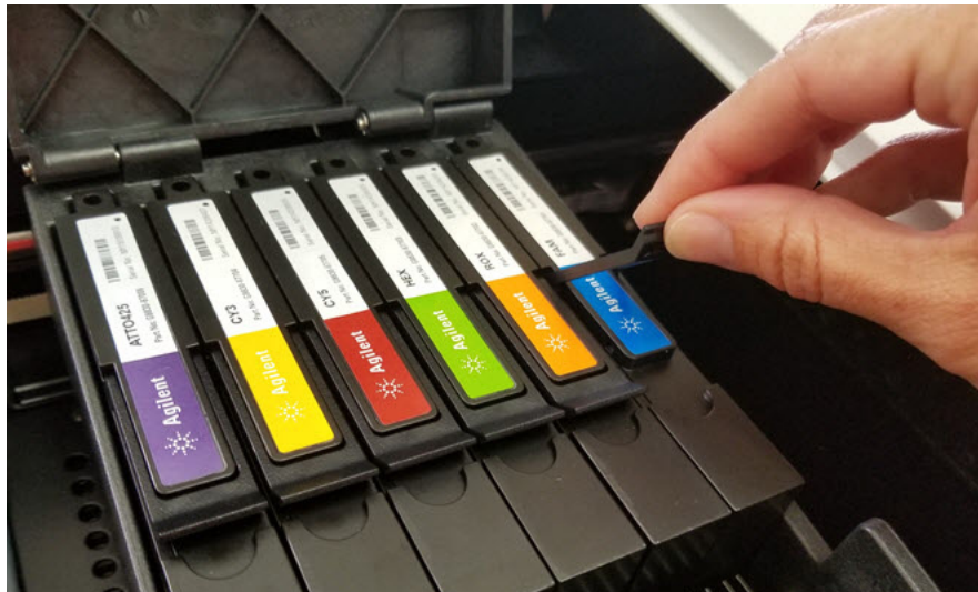
Figure 52 Lifting the hinged tab on an optical module
