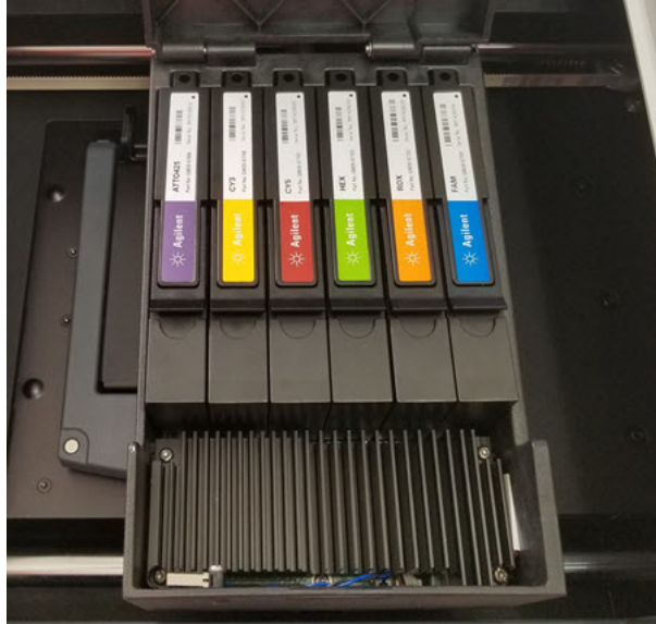
Figure 10 Installed optical modules
