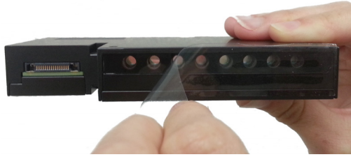
Figure 9 Removal of plastic film from optical module
